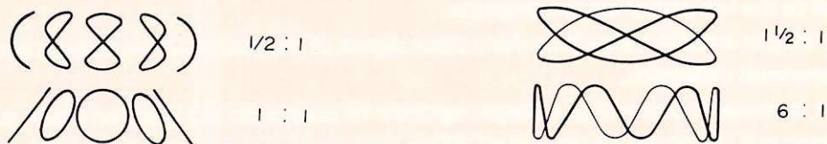
Fig. 8 Lissajous figures for frequency measurement
